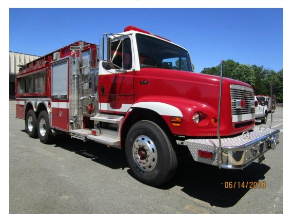
Palmetto Fire Apparatus recently took delivery of two of these sister trucks. These 2 man cab, commercial pumper tankers are unique and we don't expect them to be here for long. They both offer 2,500 gallon tanks, 1,000gpm pumps, side and rear dump chutes and an impressive amount of storage given the type of vehicle.
