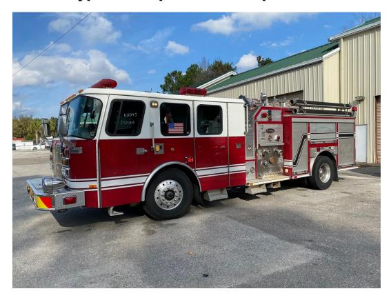
This 2005 E-One Typhoon features a rescue body with hydraulic ladder rack in a top-mount pump configuration.
