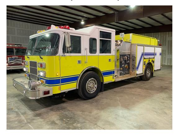
PFA0212 is a rescue pumper in a top mount configuration. Roll up doors, 1,500 gpm pump, 750 gallon tank, and a 6kW hydraulic generator.
